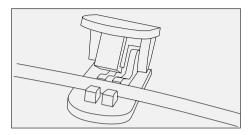
Hold the brake hose securely at the point where it should be cut.
