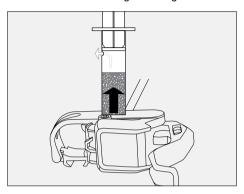
Slowly push the MAGURA Royal Blood from the filling syringe from the brake calliper into the brake system.
