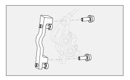
Use a 5 mm Allen key to tighten the retaining screws slightly to secure the brake calliper. It should still be possible to easily slide the brake calliper.
