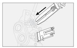
Apply the corresponding brake lever blade several times so that the brake pads are aligned and pumped against the disc brake rotor.
