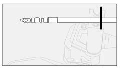
Cut the brake hose at a right angle using a suitable hose cutter (MAGURA hose cutter).
