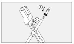
Insert a 2 mm Allen key into the front of the ETT Easy link connector. Hold the ETT Easy link connector firmly in place when screwing on the ETT sleeve nut.
