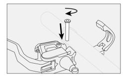
Insert the clamping screw from above through the two-part clamp into the brake lever and tighten it by turning in a clockwise direction.
