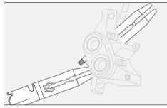
Remove the plug from the filler hole using a 3 mm Allen key. Turn it slightly back and forth. Pull out the plug while turning it.
