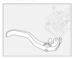
Fit the new brake lever blade. Tighten the lever pivot screw by turning it clockwise using a Torx T15 spanner.
