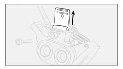
Clean the inside of the brake calliper (small brush, cloth, compressed air, etc.) with a suitable brake cleaner
