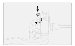
Screw in the plug of the filler hole on the brake calliper using a 3 mm Allen key and applying light pressure.
