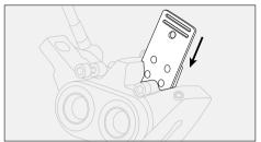
Guide the brake pad locking screw through the brake calliper and the eyelets of the brake pads.
