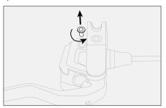
Insert the empty bleeding syringe firmly into the EBT bleed hole with a slight twisting motion.
