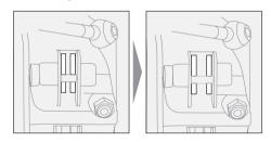
When all brake pistons are in the outermost position, release the Easy link 3 grommet on the brake lever. Push the Easy link 3 grommet onto the brake line
