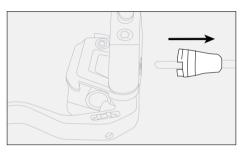
Push the ETT sleeve nut at least 5 cm onto the brake hose with the hexagon at the front.
