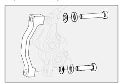
Use a 5 mm Allen key to tighten the retaining screws slightly to secure the brake calliper. It should still be possible to easily slide the brake calliper.
